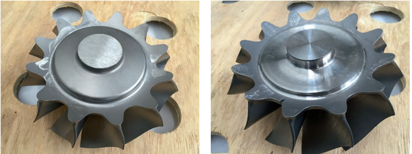
3 Turbine wheel made of Inconel 713, used for stationary gas turbines or exhaust gas turbochargers, as blank (left) and as finished part (right) (© CeramTec)
