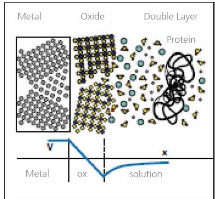
**Fig. 1** Schematic of metal-oxide-solution interface with protein molecule and voltage variations (with kind permission of L. Gilbert)
