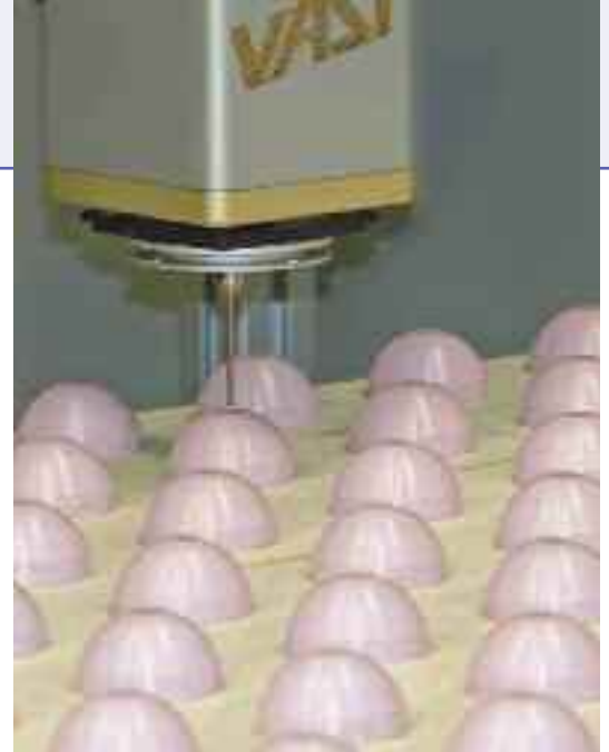
At the automatic measuring unit the data for each insert are collected online and stored in the quality module.
