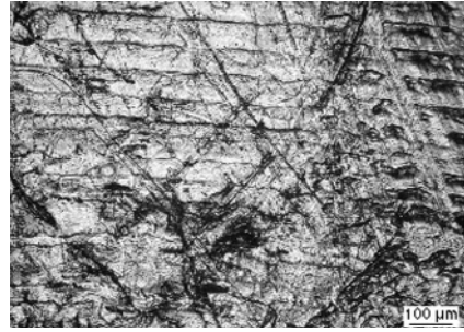
Figure 3b: Scratched Durasul Liner after 15 months in vivo.
