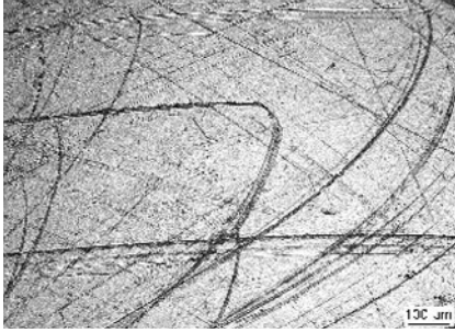
Figure 3a: Polished (worn) conventional Liner after 6 months in vivo.
